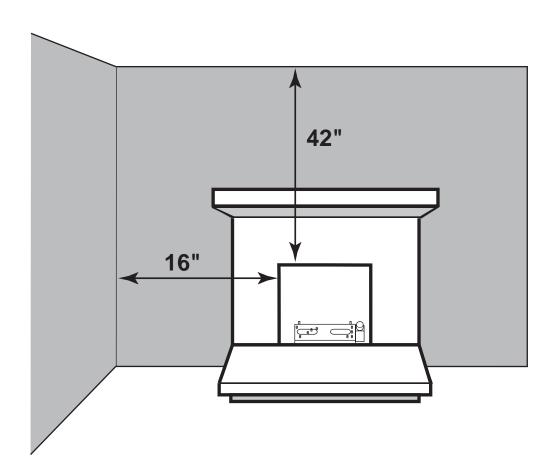
Figure 4 - Sidewall and Ceiling Clearances
